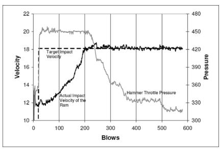
Data from the ECS - intellgient pile-driving.
